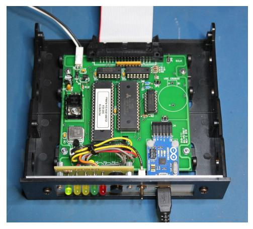
SVD-III with Remote Board installed in 3.5-inch to 5.25-inch bracket
